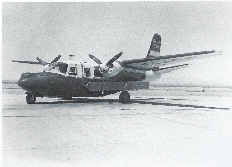
RL-27 with an APS 95 Radar installed
