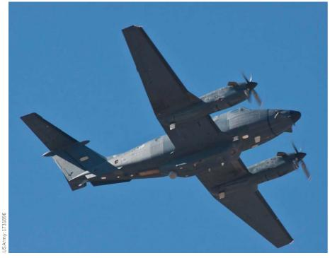
A US Army MC-12 EMARSS-M intelligence aircraft. These aircraft were converted from King Air B350 and B350ER aircraft by L3 Systems.
