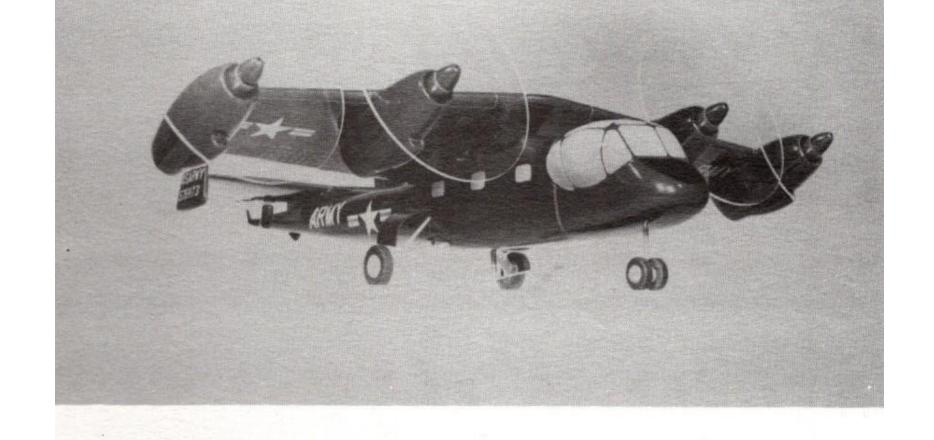
Design 134E is capable of hovering under standard loading and atmospheric conditions with only three of its four interconnected power plants operating. At overload gross weights up to 20,000 pounds, this "Super-Mohawk" requires only 240 feet to clear a 50 foot obstacle. Wing tilt angle is varied with loading for optimum short field performance.
