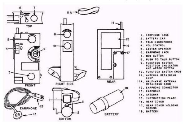
Figure 5-8.-AN/PRC-90 controls and indicators.
