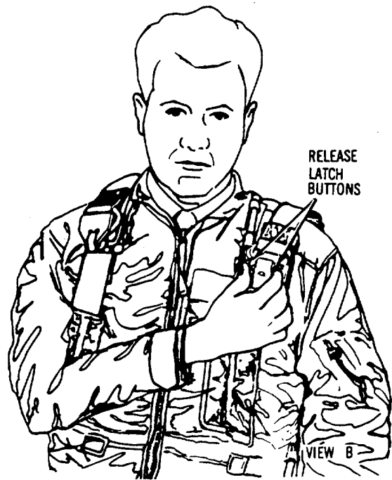
View B - Pressing latch buttons.
